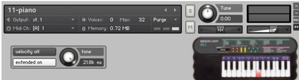
**Velocity button** - enable velocity to control volume
