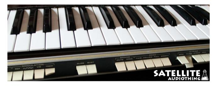
The Satellite is a rare but less known Moog synthesizer from the mid 70s. It's a monophonic preset synthesizer with one VCO and limited modulations. It was used mostly as an add-on for electric organs, in fact the US company Thomas Organ bought the license to build it. Preset sounds include brass, reeds, strings, other sounds. As many keyboards of that time the Satellite is not properly tuned along all the keys (especially at the extremes) so we included two versions: tuned and untuned.
